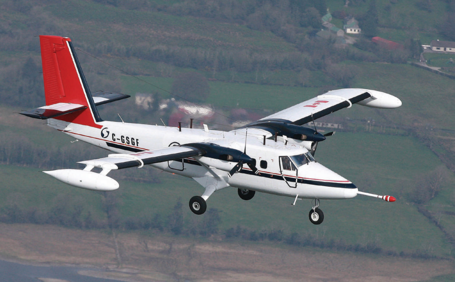
Figure 2.2. De Havilland Twin Otter survey aircraft. The wing tips contain the electromagnetic transmitter and receiver coils and one magnetometer sensor. The nose-cone houses the second magnetometer sensor.
