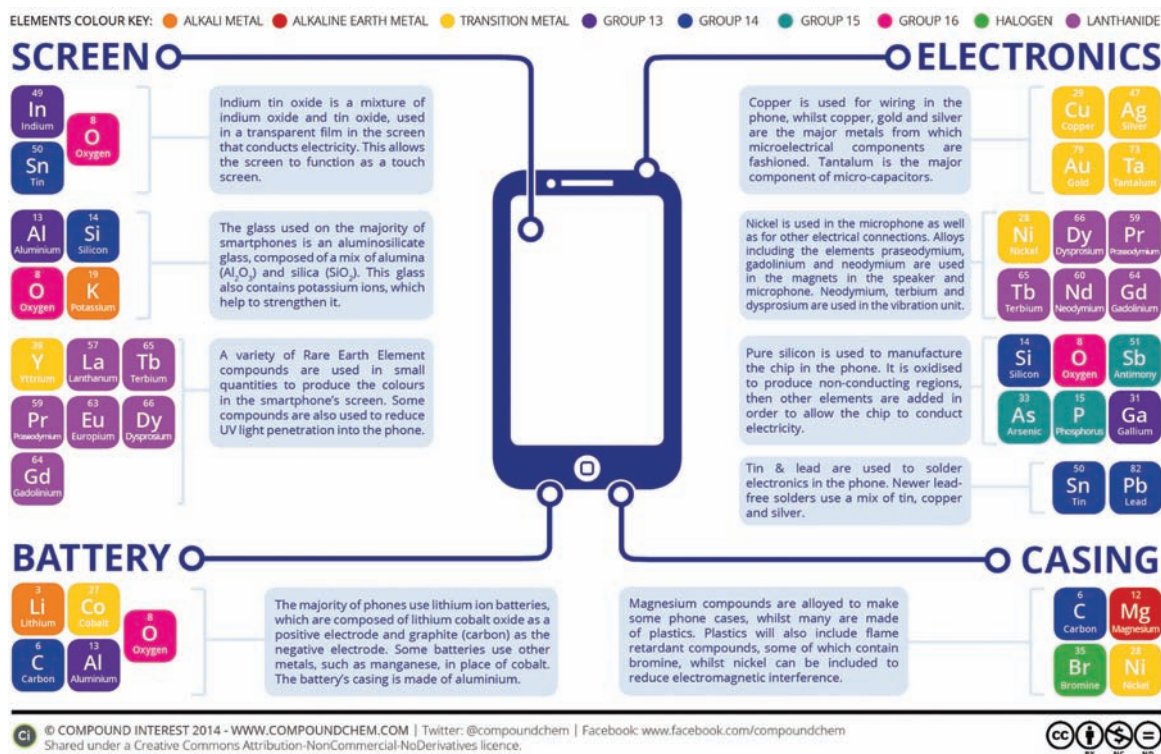
Figure 5.2 Metals contained in mobile phones (Geological Survey of Ireland (2016), Department of Communications, Energy & Natural Resources).
