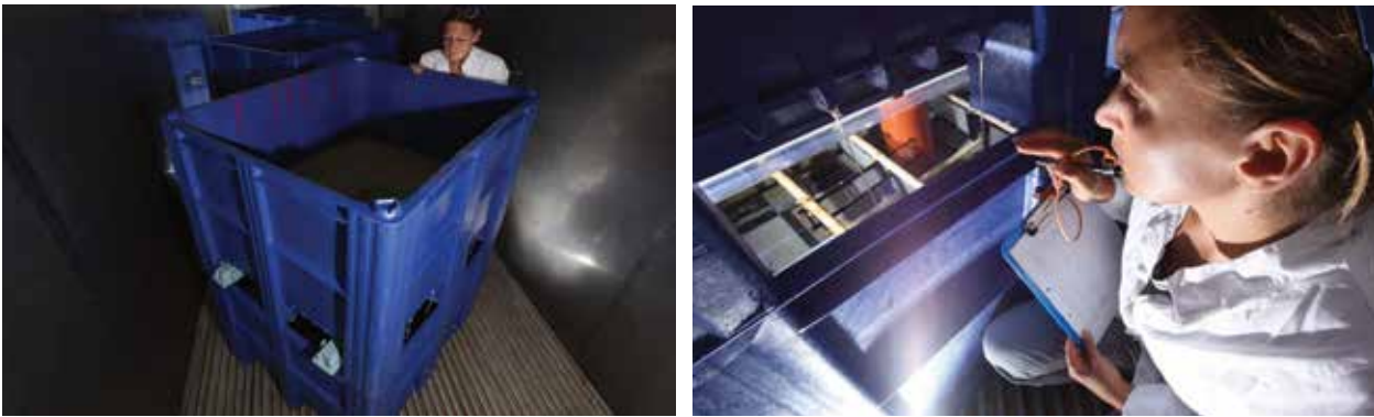
Figure 4.5: Example of a mesocosm system for testing under controlled conditions of (a) the eu littoral (intertidal), (b) sublittoral (water/sediment interface) and the pelagic (water column) habitats. (Weber et al., 2015).
